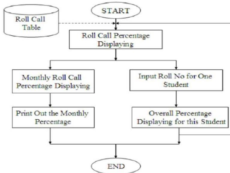
Figure 11: Flowchart of the Roll Call Percentage Displaying
