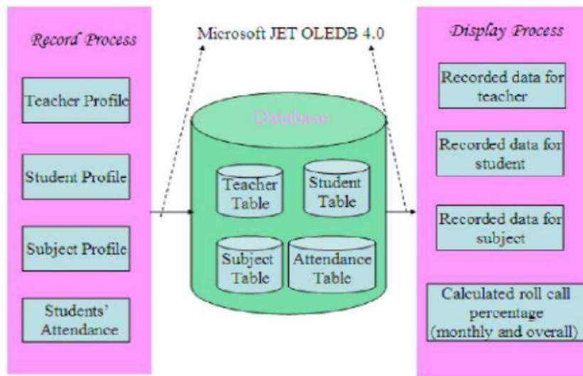
Figure 3: Overall Block Diagram of the System
