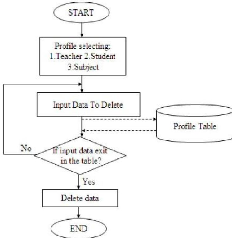
Figure 9: Flowchart of the Profile Delete
