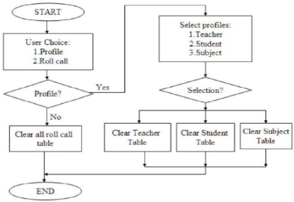
Figure 12: Flowchart of the Clearing Table
